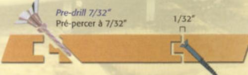
To screw planks into the tongue and groove, pre-drill 7/32" diameter holes, countersink holes and use 2" length #8 galvanized or stainless steel flat-head wood screws. Leave a space of 1/32" between each plank (approximately the thickness of a dime).
