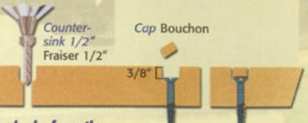
To screw planks from the surface, use 2" length #8 galvanized or stainless steel flat-head wood screws.
